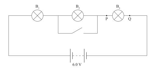
(c) When the switch is **open**, the current through the circuit is **0.40A**.
