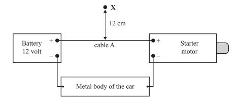
The starter motor is turned on and a large current flows through cable A. The power output of the motor is 540 W. The point X is 12 cm from cable A.
