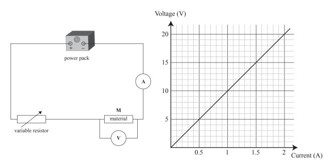
The above graph shows how the current through the conducting material changes as the voltage across it varies.
